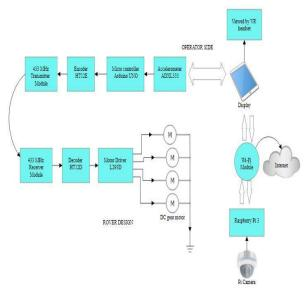
Figure 1.Block Diagram of the proposed model
