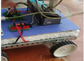
Figure 10. Rover Design in which RF receiver receives the signals which is then given to the motor driver L293D which is in turn connected to four dc motor for the robot movement.
