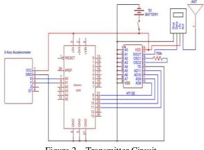
Figure 2. Transmitter Circuit
