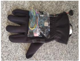
Figure 9. Transmitter Design in which the accelerometer sensors the movement and feds signals to the Arduino UNO microcontroller.
